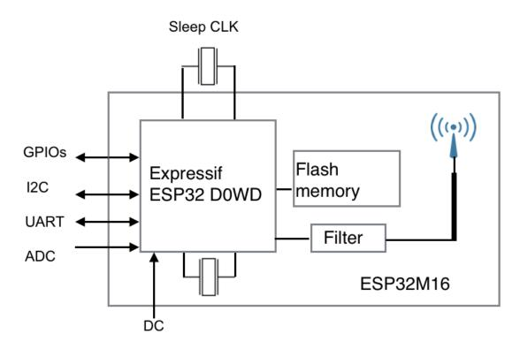
There are two CPU cores that can be individually controlled, and the CPU clock frequency is adjustable from 80 MHz to 240 MHz. The main CPU can be powered off and use the low power co-processor to constantly monitor the peripherals for changes or crossing of thresholds. ESP32 integrates a rich set of peripherals, ranging from capacitive touch sensors, Hall sensors, SD card interfaces, Ethernet, high-speed SPI, UART, I<sup>2</sup>S, and I<sup>2</sup>C.
